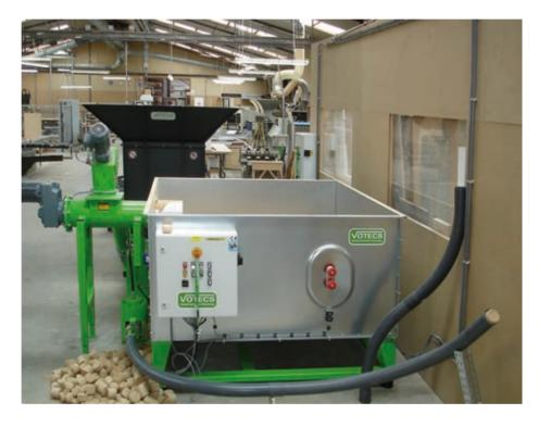
Depending on the material, the briquetting press "AP 775" enables hourly capacities of 120 to 160 kg.
