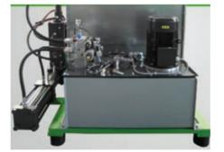
The hydraulic tank is arranged separately. In this way, the emerging oil heat is optimally discharged. Easy access makes the regular maintenance service pleasant and efficient.
